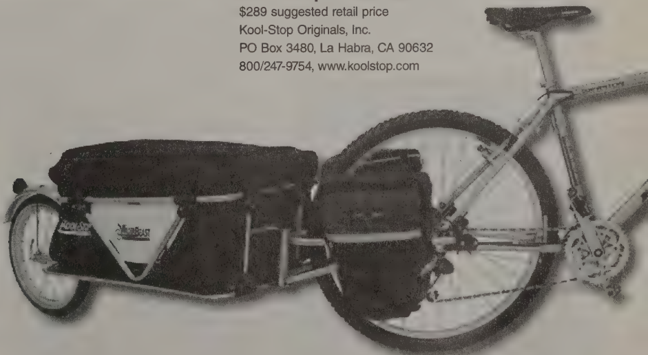
The Wilderbeast in action. 100-percent Chrome-Moly with a weight capacity of 70 lbs; it's highly maneuverable and doesn't interfere with riding the bike.
